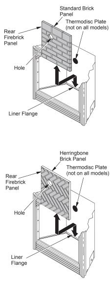
Figure 3 - Placing Rear Firebrick Panel on Flange in Fireplace
